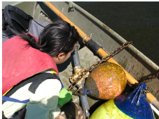
Below: Example of bio-fouling on continuous monitors deployed in Upper Klamath Lake
